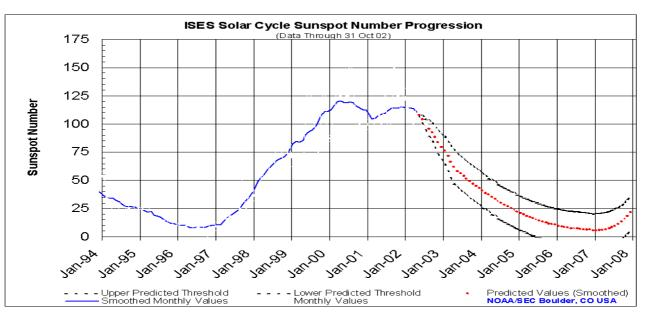
The diagram shows the progression of the current solar cycle, with the prediction for the next minima being around June 2007. The "double hump", or twin peak can be clearly seen. Expect conditions to deteriorate steadily over the next few years.
