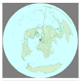
The England – New Zealand path as shown on a great circle map (notice that it is a straight line and crosses over the North Pole). If an aircraft were to fly direct from the UK to New Zealand, this would be the preferred route as it is the shortest or **SHORT PATH**. Most radio communication on the HF bands is conducted via Short Path.
