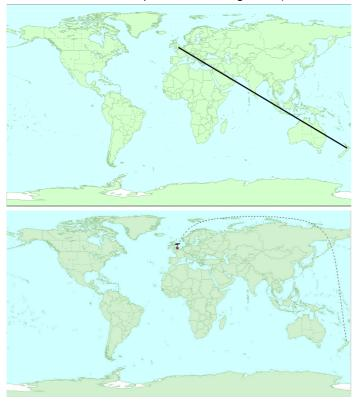
Mercator projection) will give you false information as to how the radio wave reaches it's target. To get the true picture you need to look at a globe or a special type of map called a '**GREAT CIRCLE**', which is a representation of the globe if it were flattened onto a piece of paper.
